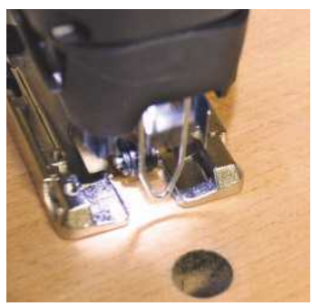
▲ A trigger-activated LED gives good vision around the work area
